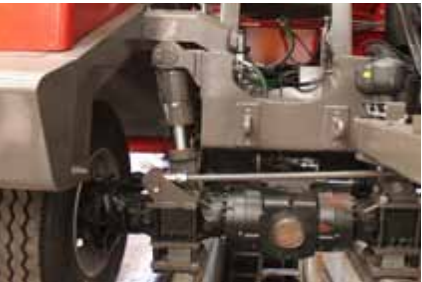
Rigid construction chassis with front and rear hydraulic suspensions.
