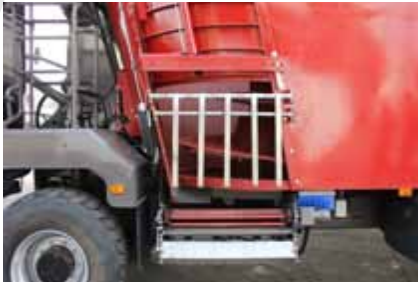
Adjustable discharge conveyor on LH driver's side made from 3CR12 with C55 chain.
