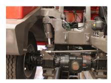
Rigid construction chassis with front and rear hydraulic suspensions.
