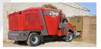
Front loading elevator equipped with rubber belt 650mm width, Quick, efficient, precise and homogenous mixing - preserving the nutritional value.
